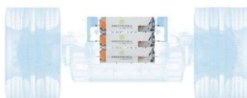
H1 TRIPLE-STACK WITHIN FRAME RAILS
